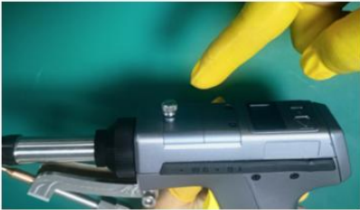
① Unscrew the protective lens screw
